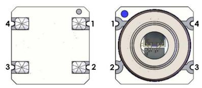
Figure 13: pin configuration
