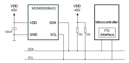
Figure 12: Typical application circuit with I<sup>2</sup>C protocol communication
