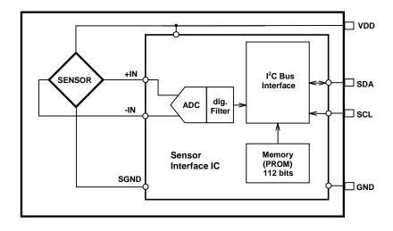
Figure 1: Block diagram of MS5805-02BA
