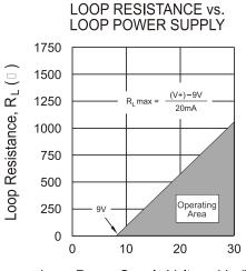
Loop Power Supply Voltage, V<sub>PS</sub>(V)
