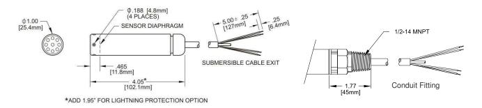
**Gland Cable Seal Configuration for ETFE Cable**
