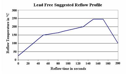
Mount parts within 24 hours after printing solder paste to avoid potential dry up.
