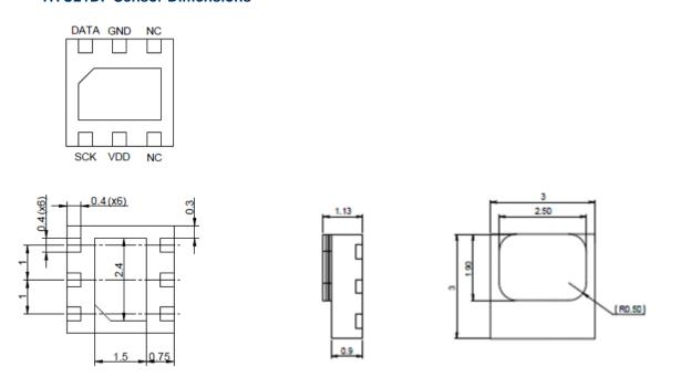
Dimensions are given in mm, tolerances are  $\pm 0.1$ mm. The die pad (thermal center pad) is internally connected to GND.
